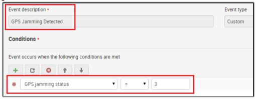
Figure 1: GPS Jamming Detected Event
