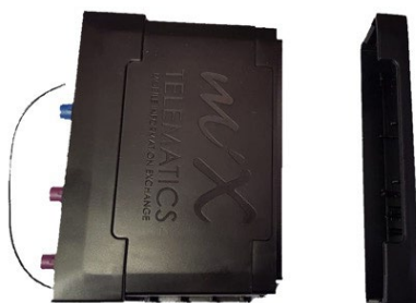
Figure 2: Unhook the cover
