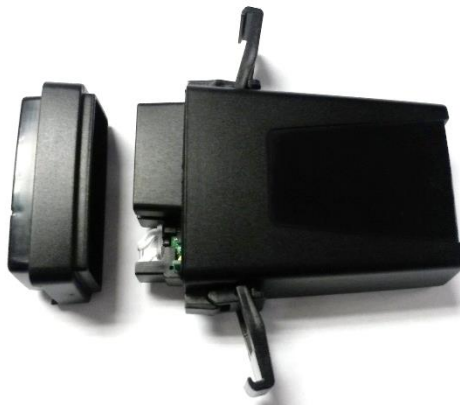
Figure 4 Remove outer faceplate
