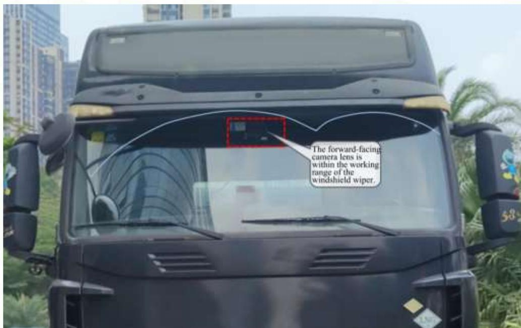
Figure 28: Main unit installation position.
