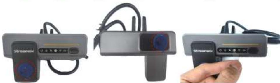
Figure 16: Removing protective stickers and film
