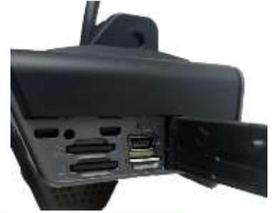
Plug USB in [Mini USB OTG Adaptor](#) and then in the powered up unit. The FW upgrade process will start and take about 6min.
