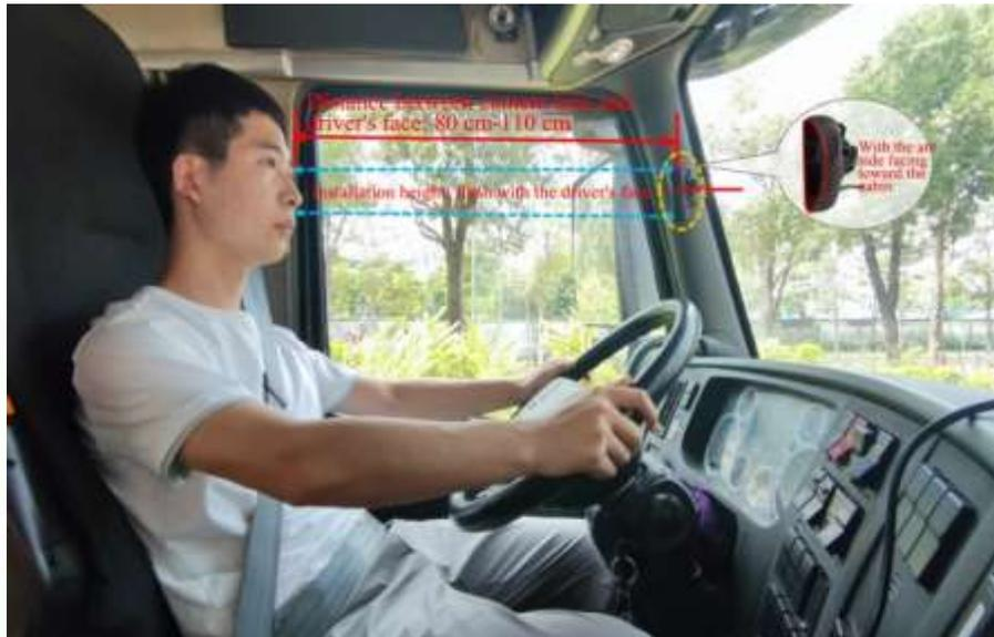
Figure 47: A-Pillar mount installation
