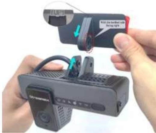
Figure 31: attaching the main unit to the bracket.
