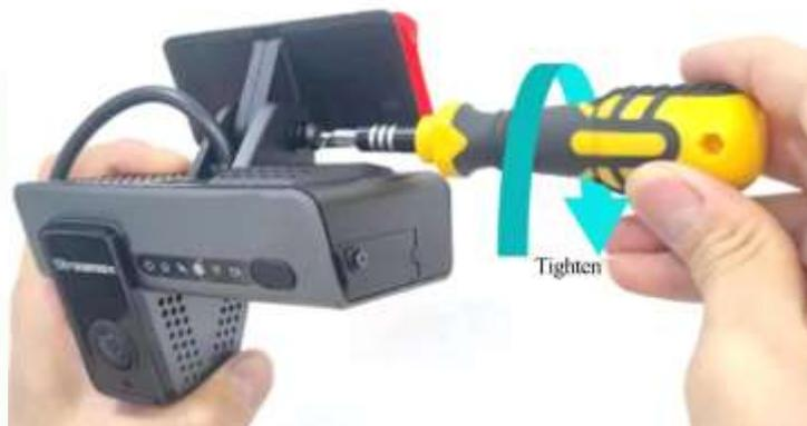
Figure 32: fixing the main unit to the bracket.
