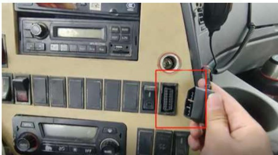
Figure 38: Connecting to the OBD port.
