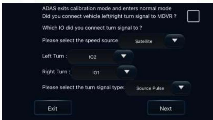
Figure 80: Configure Left/Right turn indicators.
