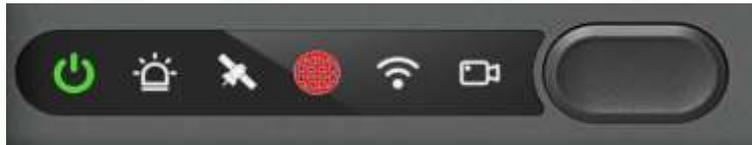
Figure 110: MiX Vision AI LED panel indicating Flight Mode.
