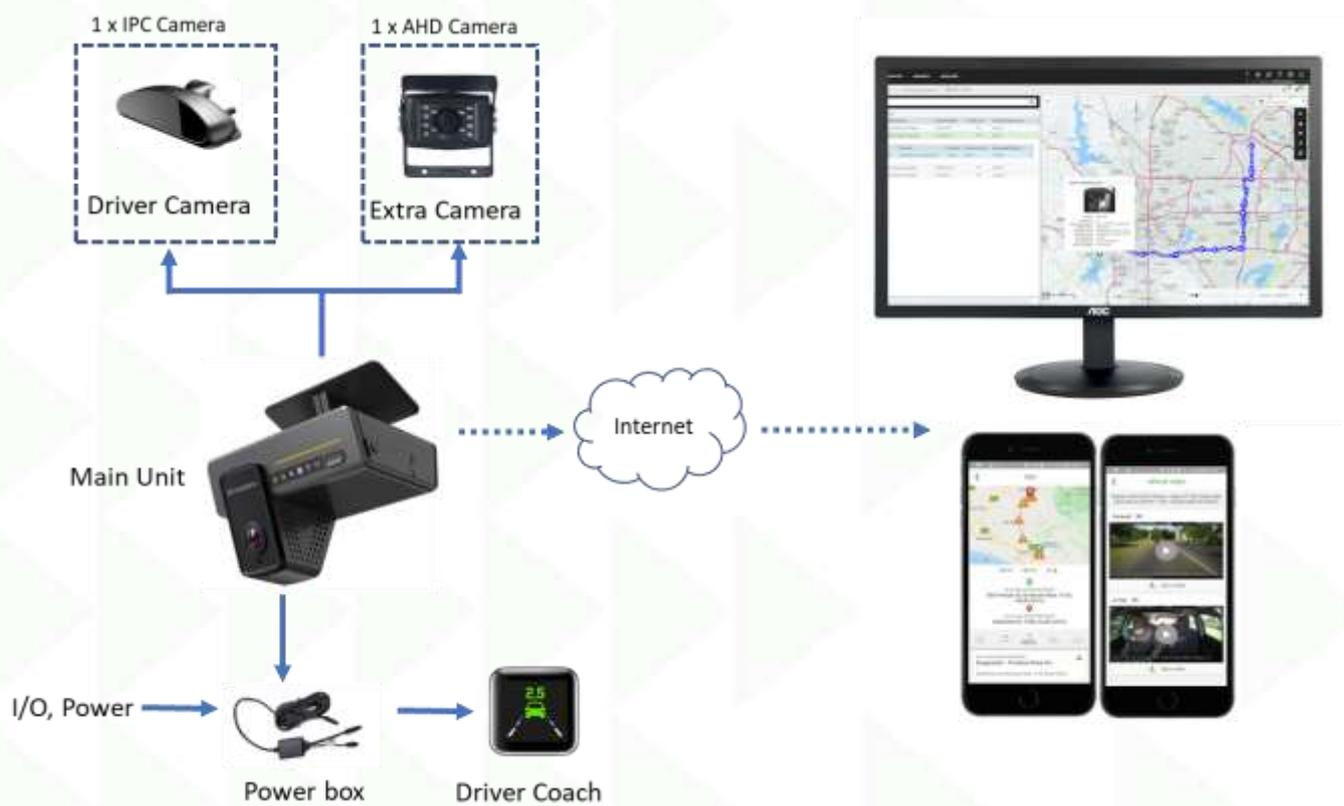
Figure 5: System Diagram.
