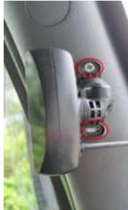
Figure 50: Tighten the upper screw of the DSM camera mount
