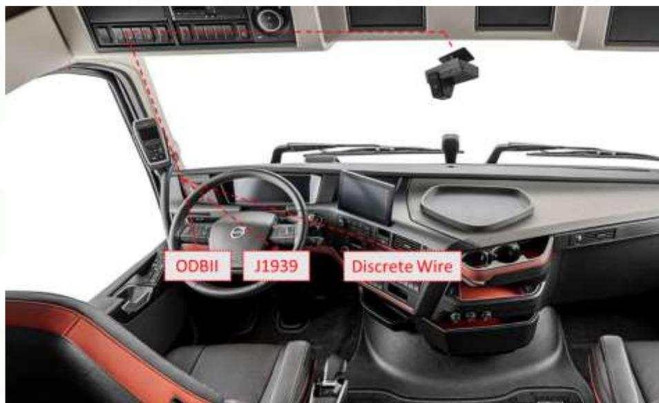
Figure 34: Locations for the vehicle's connections.
