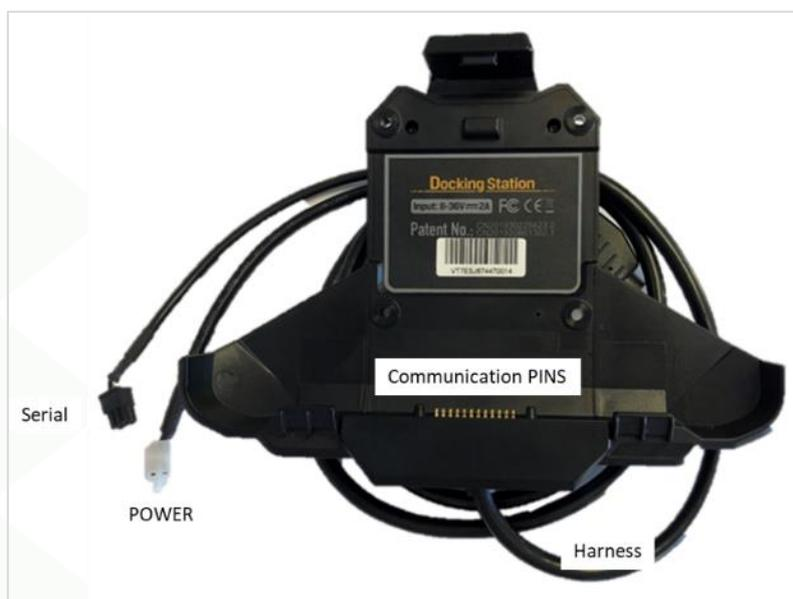
**Figure 5: Rovi IV Docking Station – Front**
