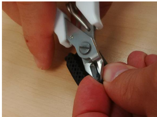
Figure 7 Cut hole in rubber
