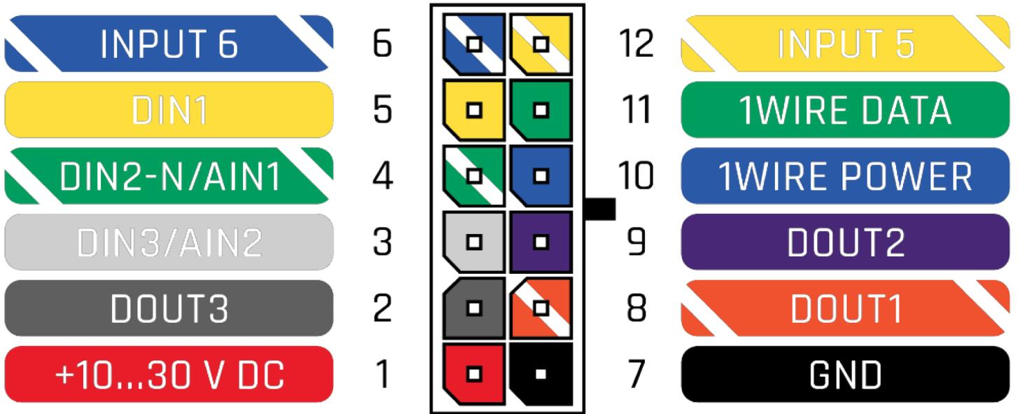
Figure 2 device 2x6 socket pinout
