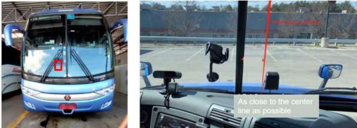
Figure 16: Installation location if wiper rests in the middle of the windshield.
