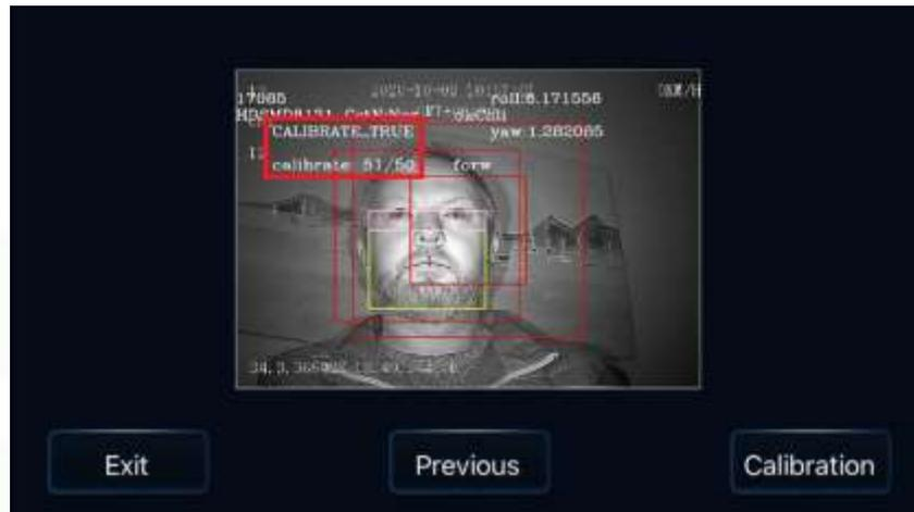
Figure 57: Driver camera calibration (Dash Mount).
