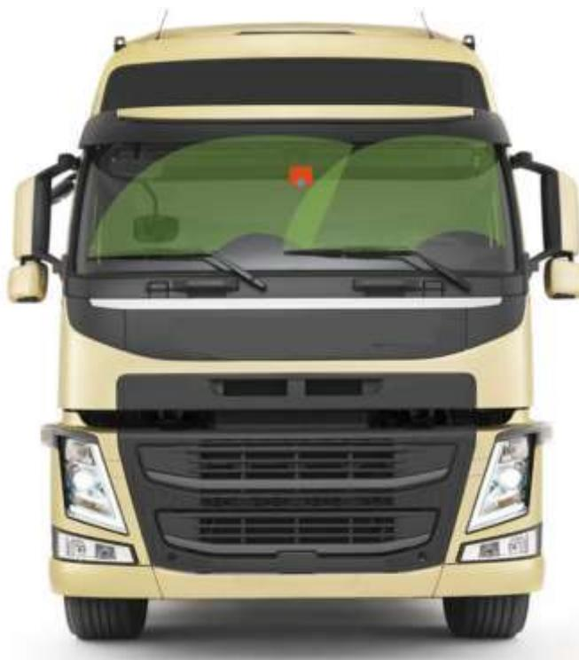
Figure 14: Main unit installation location
