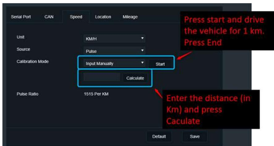
Figure 59: Speed Calibration.
