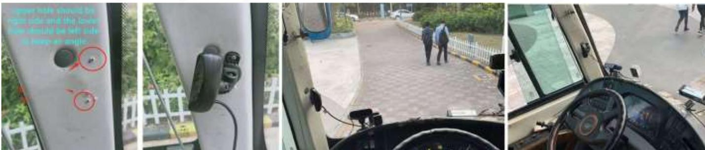
Figure 24: Example A-Pillar mount installation
