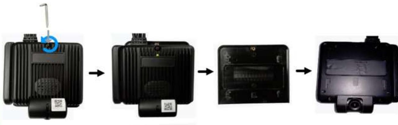
Unscrew the screw on the top. The screw is fixed to the main unit.
