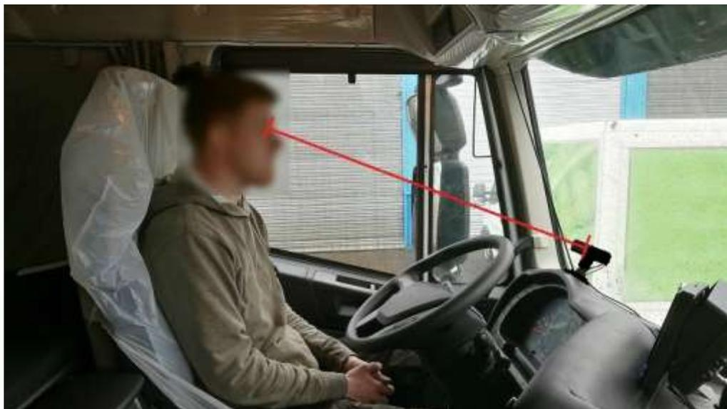
Figure 22: Correct Driver Camera Installation.
