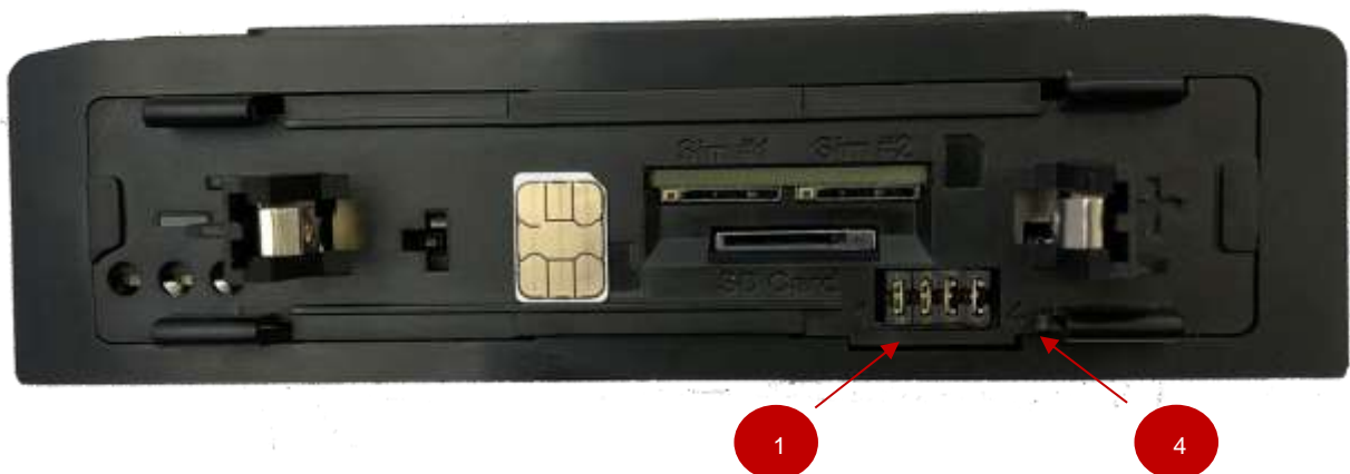
Figure 7: Position of jumpers on the PCB (viewed from the back)
