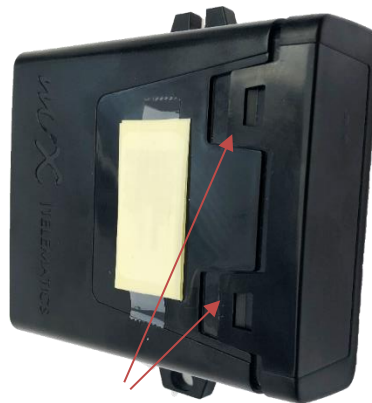
Figure 1: Opening of side clips
