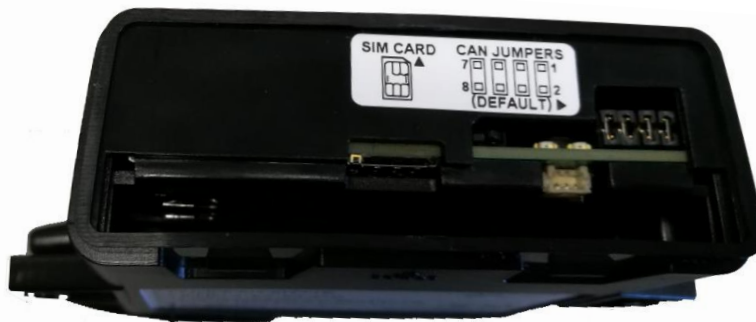
Figure 7: Position of jumpers on the PCB.
