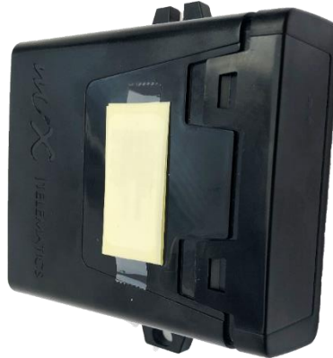
Figure 5: Clip the cover back on; the hooks need to click into place.
