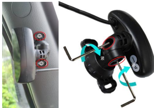
Figure 53: Tighten the lower screw of the DSM camera mount
