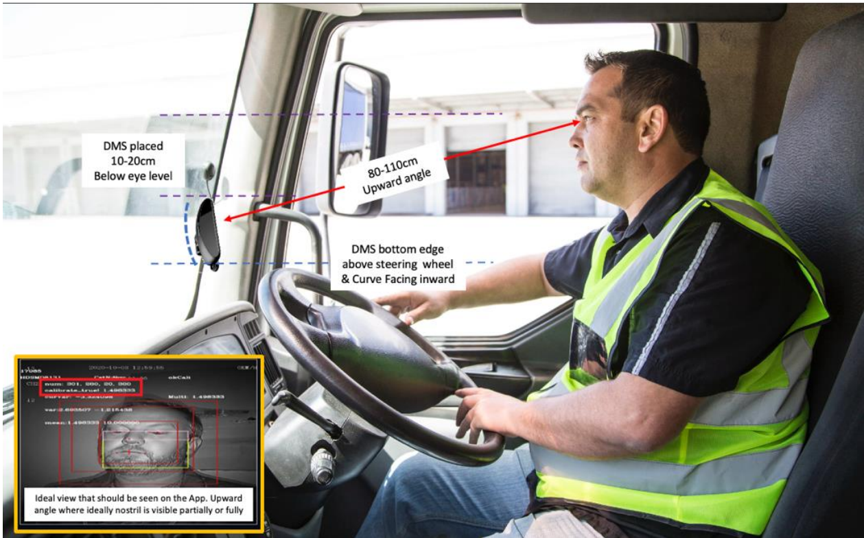
Figure 47: A-Pillar mount installation
