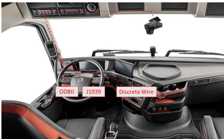
Figure 34: Locations for the vehicle's connections.
