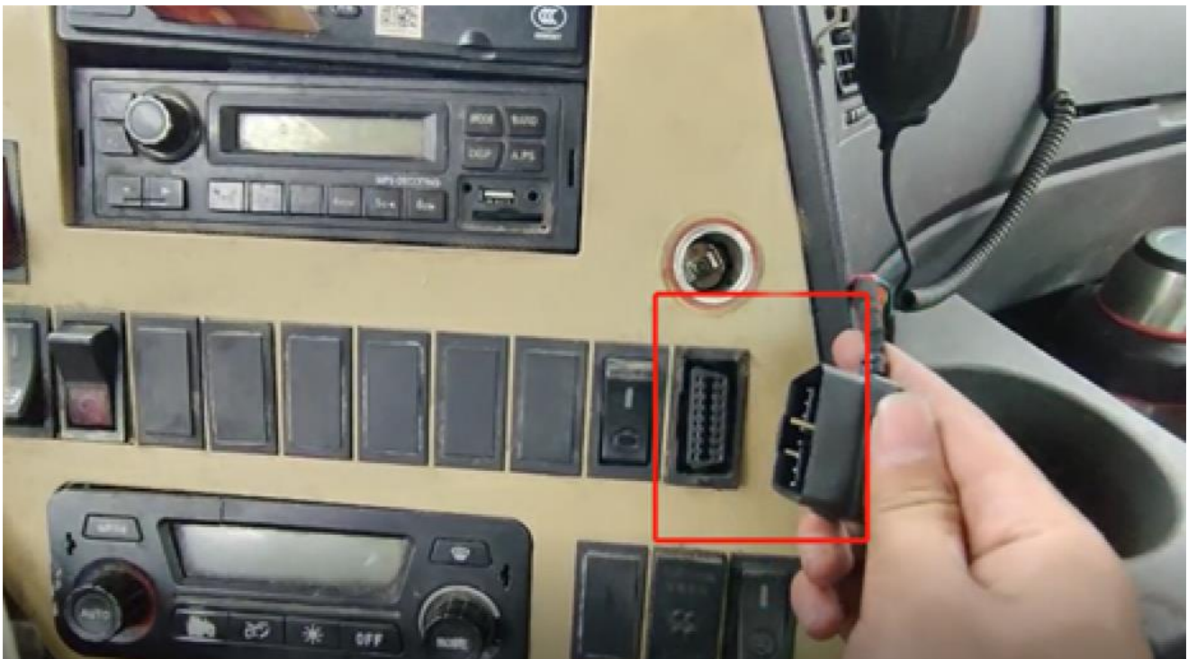
Figure 38: Connecting to the OBD port.
