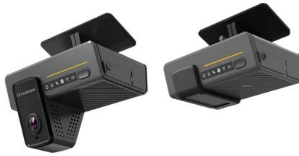
Figure 2: VisionAI (AD Plus 2.0) and AD Plus2.0-S Main Device.
