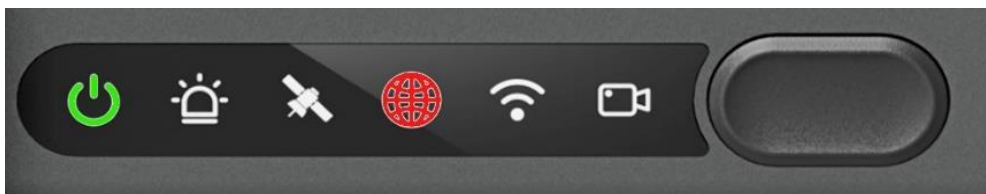
Figure 3: VisionAI LED panel indicating Flight Mode.
