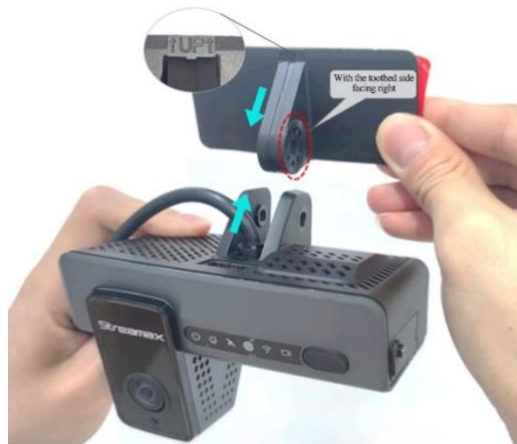
Figure 31: attaching the main unit to the bracket.
