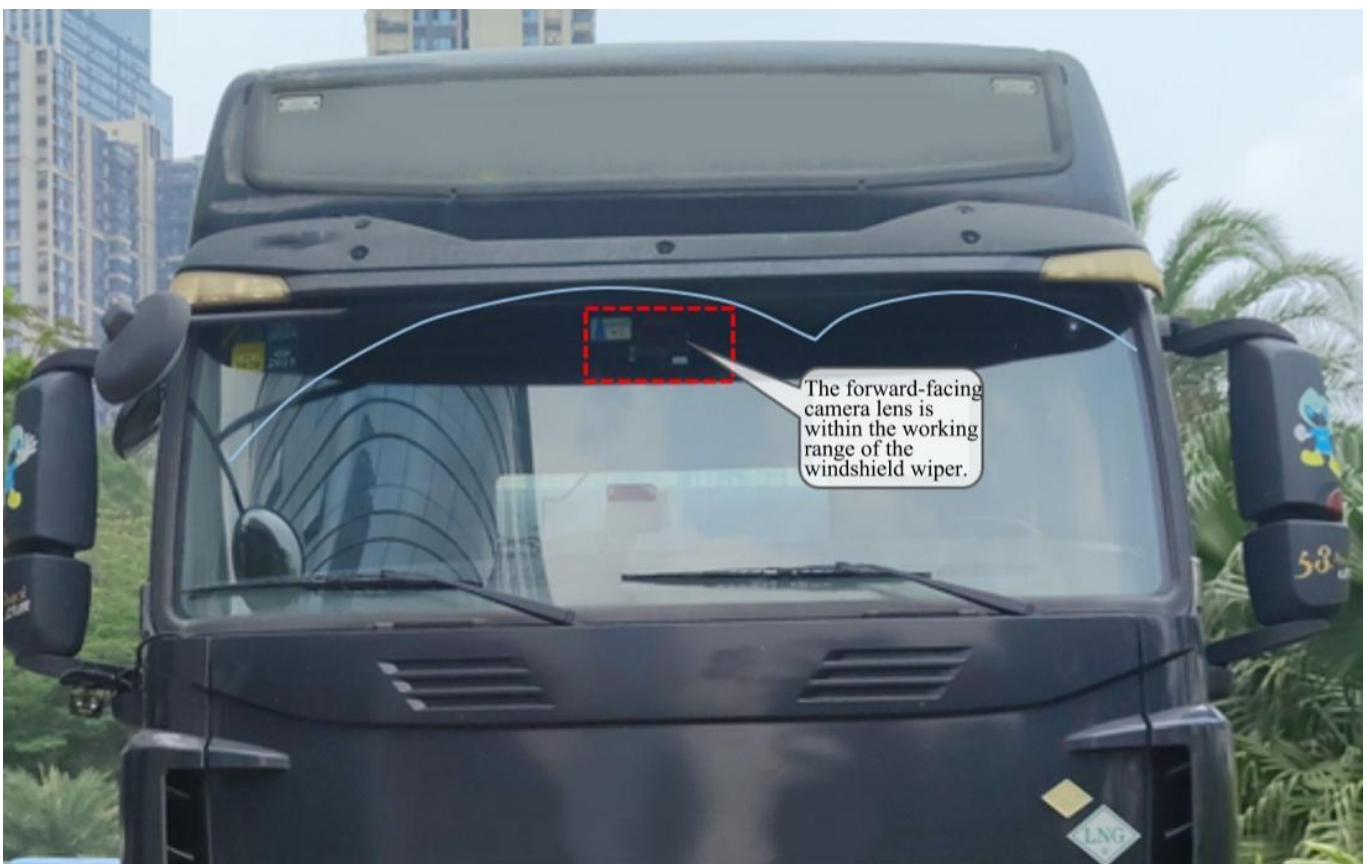
Figure 28: Main unit installation position.
