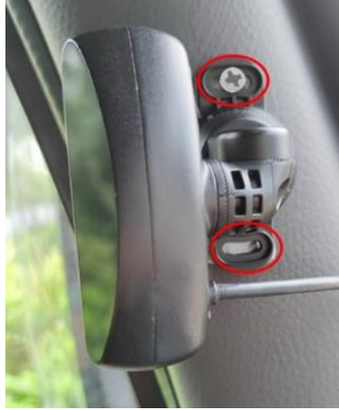
Figure 50: Tighten the upper screw of the DSM camera mount
