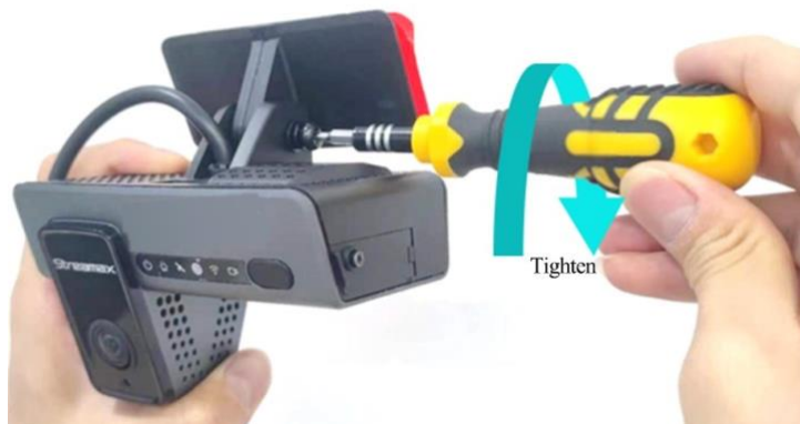
Figure 32: fixing the main unit to the bracket.
