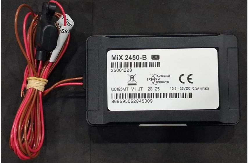
A photograph showing the MiX 2450-B LTE Consumer Electronic Unit. The unit is a black rectangular device with a white label on its front. The label displays the text 'MiX 2450-B LTE', a barcode, the serial number '25001028', and regulatory information including 'TA-2024/3465', 'CLASS A APPROVED', 'CE', 'U0195MT V1 JT 28 25 10.5-33VDC; 0.5A (max)', and the number '869595062845309'. A power harness with red and brown wires is coiled and attached to the back of the unit. |
