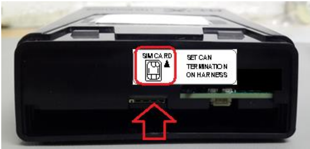
Figure 3: Position the SIM as shown on the unit.
