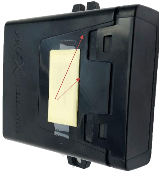
Figure 1: Opening of side clips
