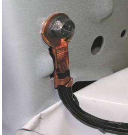
*Figure 12 - Connecting negative power wire*
