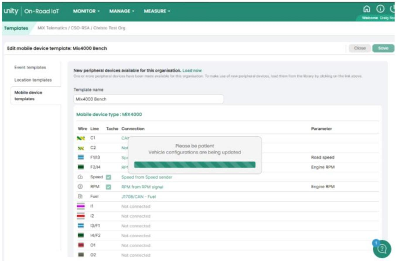
Select the serial port which RIBAS is connected to, either S1 or S2 and click on “Not connected”
