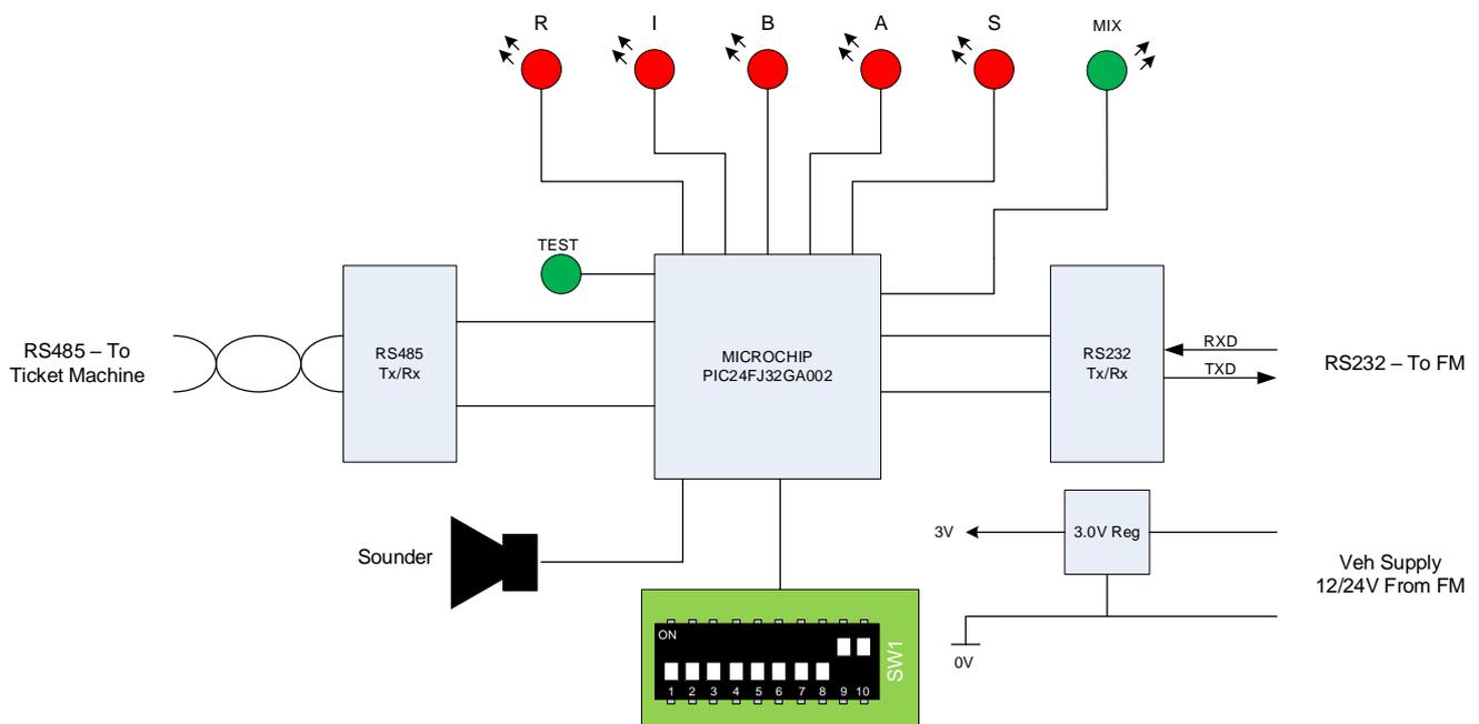
The RIBAS™ design simply provides a microprocessor between 2 serial interfaces. The RS232 connects to the MiX4000 OBC (power is also provided by the OBC) and the RS485 connects to the ETM.
