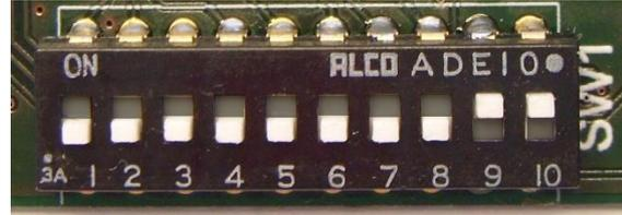
Figure 1 - Switch 0-8 off 9 -10 on (Normal RIBAS™ setting) down (0) = off, up (1) = on
