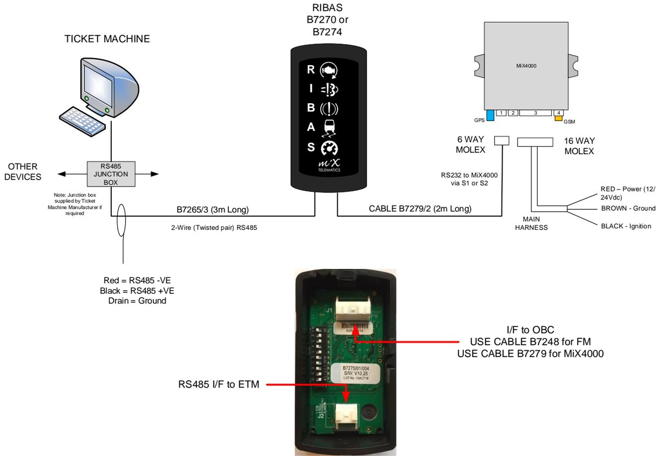
The setup shown above is typical of a bus installation where RIBAS™ interfaces to a ticket machine (ETM) via the RS485 interface. The switch settings on the DIP switch will determine the protocol for the RS485 comms to the ETM.
