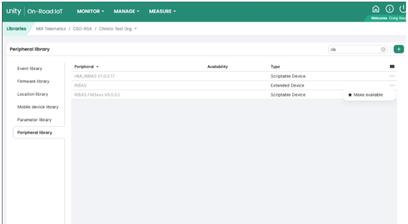
If the RIBAS Extended Device is greyed out, make it available by clicking on the 3 dots to the right of the device and select Make Available.
