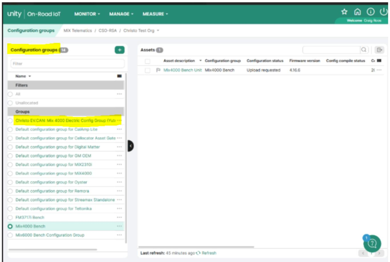
Click on the green Mobile Device Template (Mix4000 Bench in the example below) – modifications to the device should be made at the template level.
